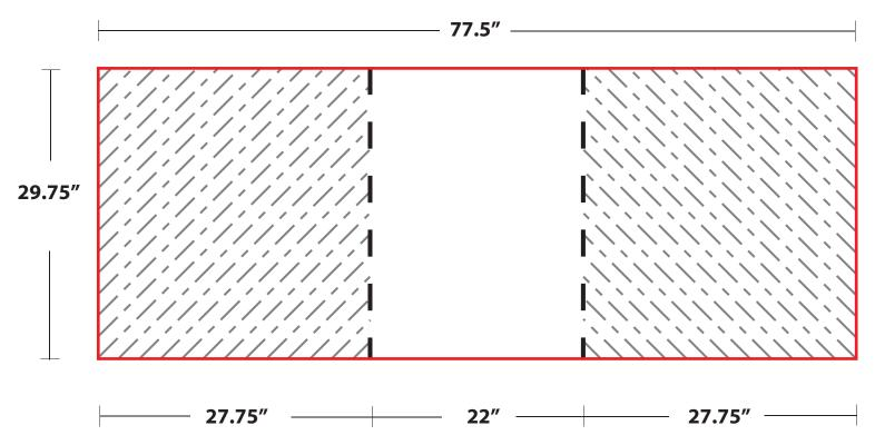
\*The hatched area is the area that wraps around the sides and behind the case, and is not visible from directly in front.
